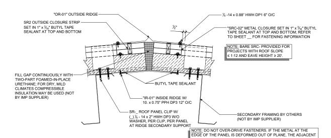
PANEL WILL BE DIFFICULT TO ENGAGE AND WILL NOT SEAM. AFTER SR CLIP HAS BEEN INSTALLED OVER MALE LEG OF STANDING SEAM
