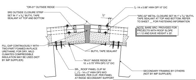
NOTE: DO NOT OVER-DRIVE FASTENERS. IF THE METAL AT THE EDGE OF THE PANEL IS DEFORMED OUT OF PLANE, THE ADJACENT PANEL WILL BE DIFFICULT TO ENGAGE AND WILL NOT SEAM. AFTER SR CLIP HAS BEEN INSTALLED OVER MALE LEG OF STANDING SEAM PANEL, PRE-CRIMP, USING ½" HAND CRIMPING TOOL.
