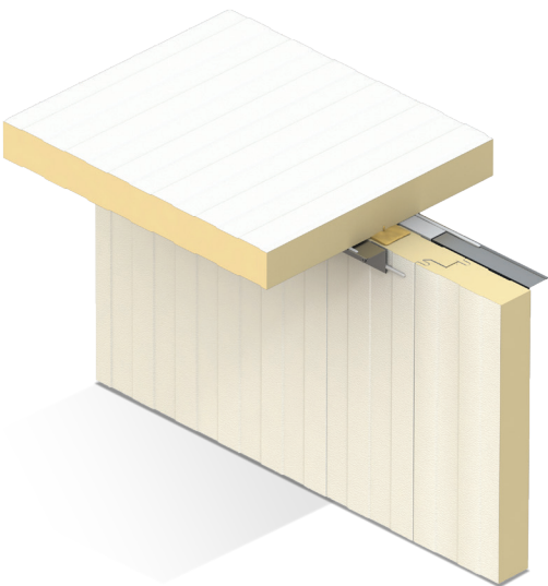
Wall to Ceiling Intersection
