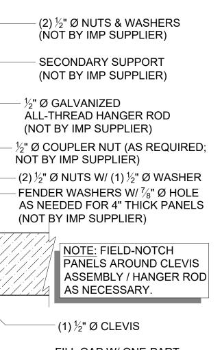
FILL GAP W/ ONE-PART EXPANDING FOAM SEALANT (NOT BY IMP SUPPLIER)
