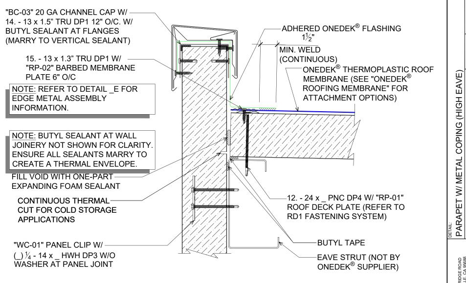
BASE FLASHING AT PARAPET W/ METAL # COPING (HIGH EAVE)
