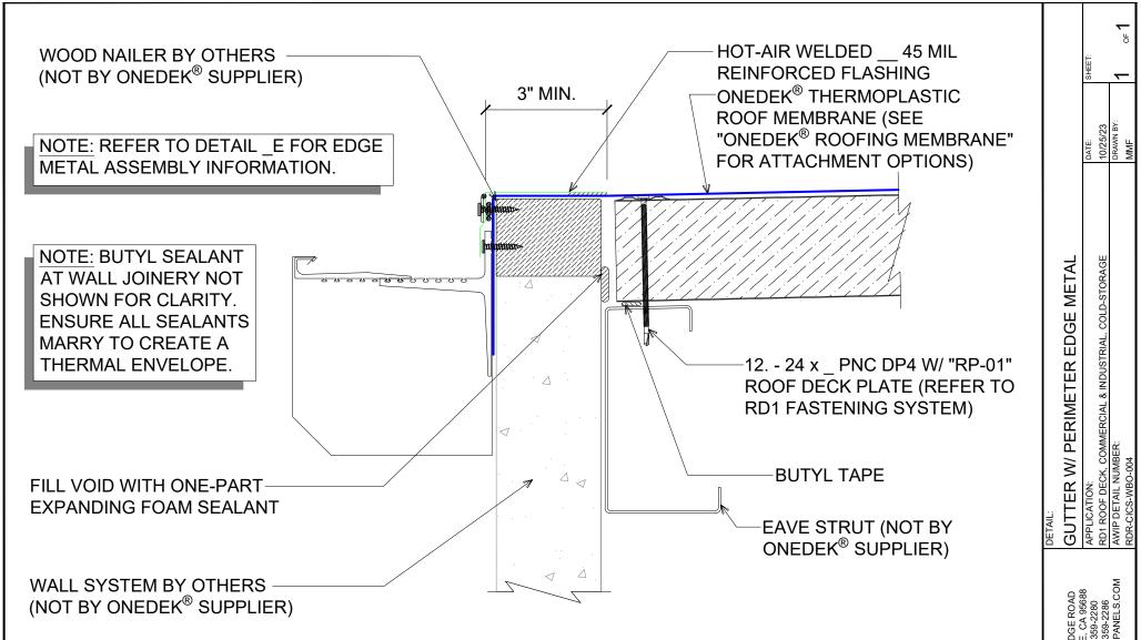
**GUTTER W/ PERIMETER EDGE METAL** #
