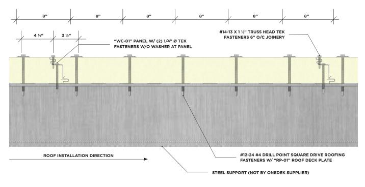
RD1/RD1-M DIAPHRAGM FASTENING SYSTEM (40/7-6) (SECTION VIEW)
