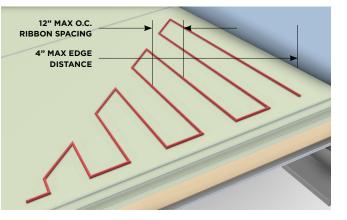
Mechanically attached membranes are used with mechanically attached tapered insulation systems and where fully adhered membranes are used with adhered tapered insulation systems. AWIP currently doesn't offer the combination of fully adhered membranes with mechanically attached tapered insulation.
