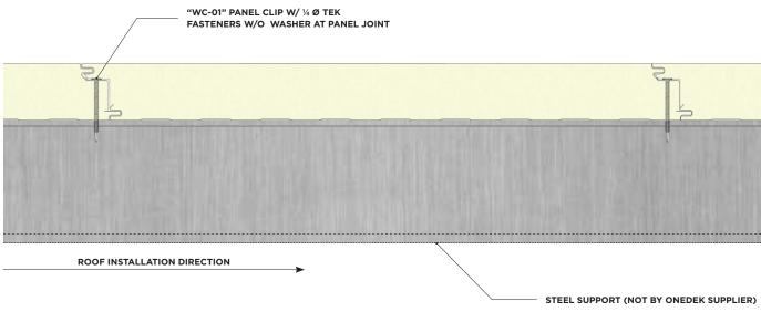
• This fastening system does not provide any diaphragm resistance.
