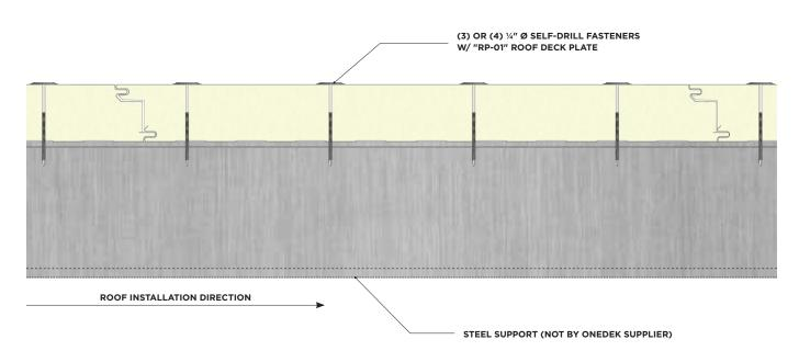
**RD1/RD1-M NON-DIAPHRAGM THROUGH FASTENING** (SECTION VIEW)
